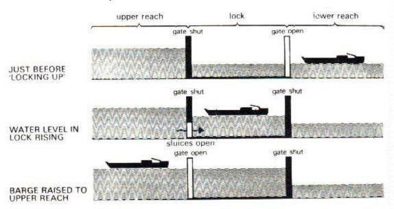
Using a system of gates on a hill the canal builder could create a system where-by the people working the barge could open and shut gates in the order demonstrated above to move the barge uphill.
